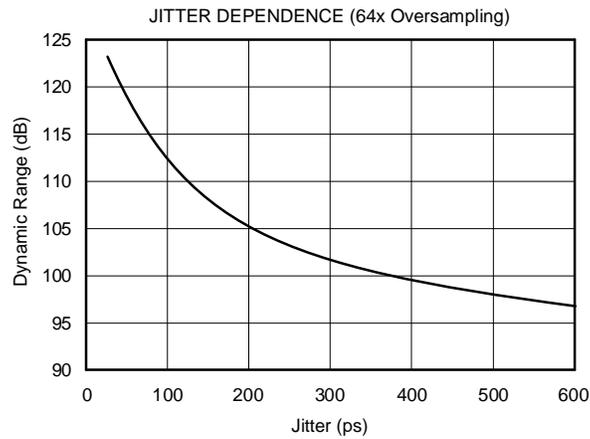
**Figure 34. Jitter Sensitivity**
