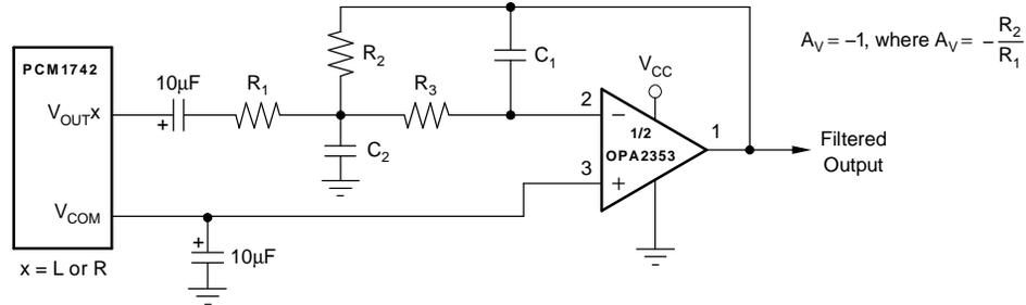
(a) Using V<sub>COM</sub> to Bias a Single-Supply Filter Stage
