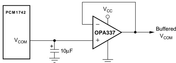
(b) Using a Voltage Follower to Buffer V<sub>COM</sub> When Biasing Multiple Nodes
