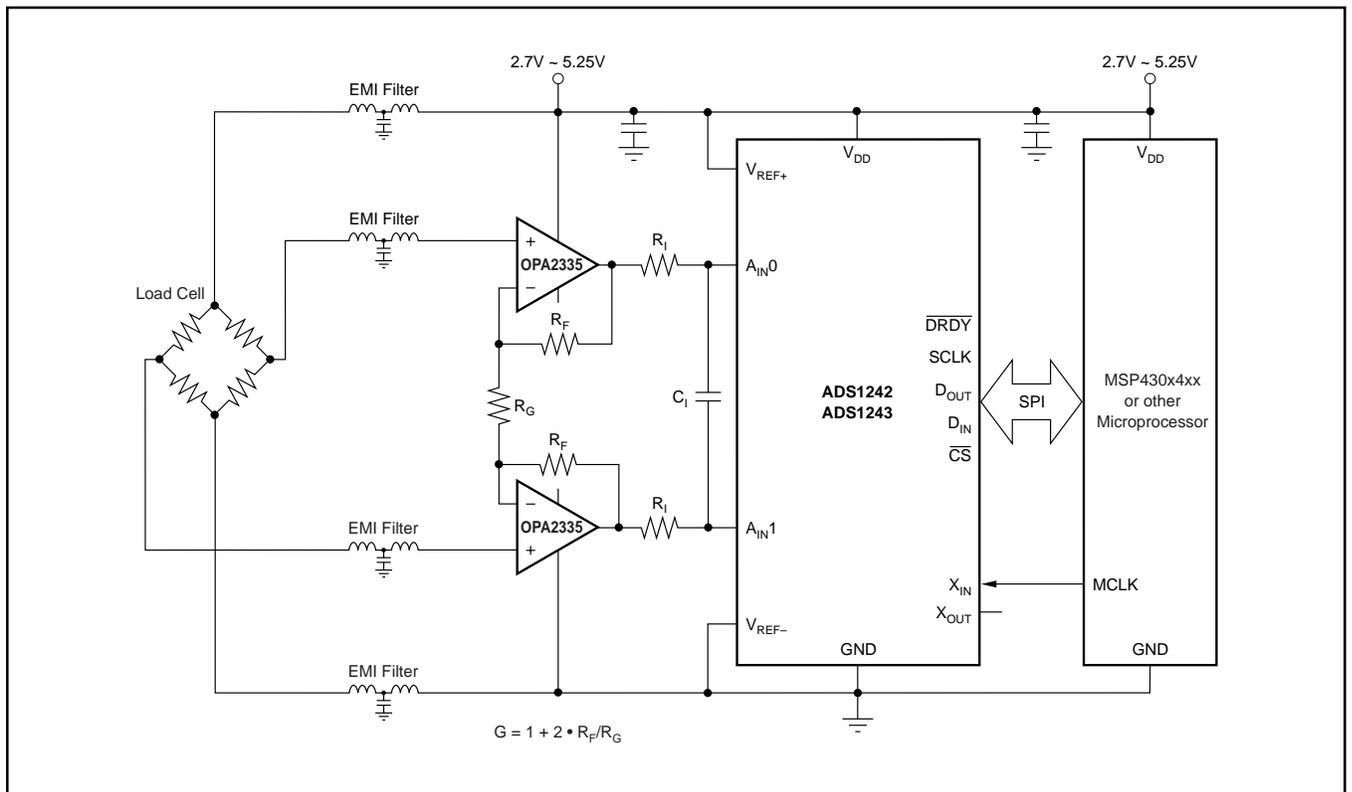
FIGURE 9. Block Diagram for a High-Precision Weight Scale.
