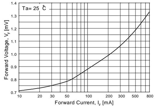
Figure 6. Forward Voltage vs Forward Current
