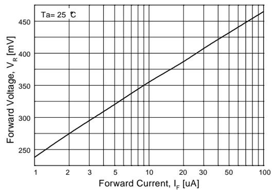
Figure 4. Forward Voltage vs Forward Current
