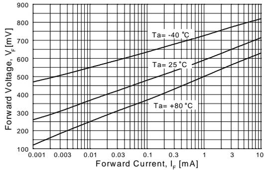
Figure 7. Forward Voltage vs Ambient Temperature
