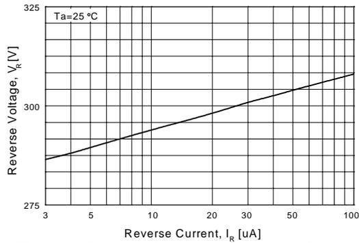
Figure 1. Reverse Voltage vs Reverse Current
