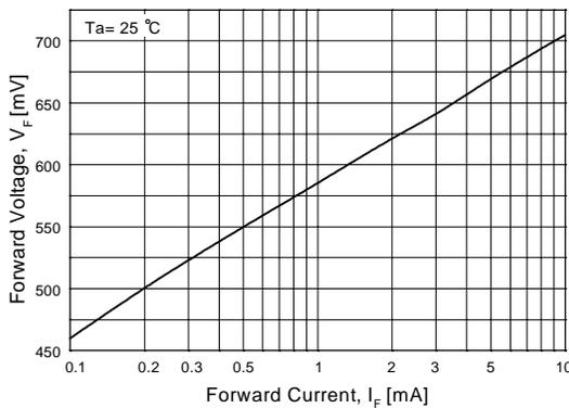
Figure 5. Forward Voltage vs Forward Current
