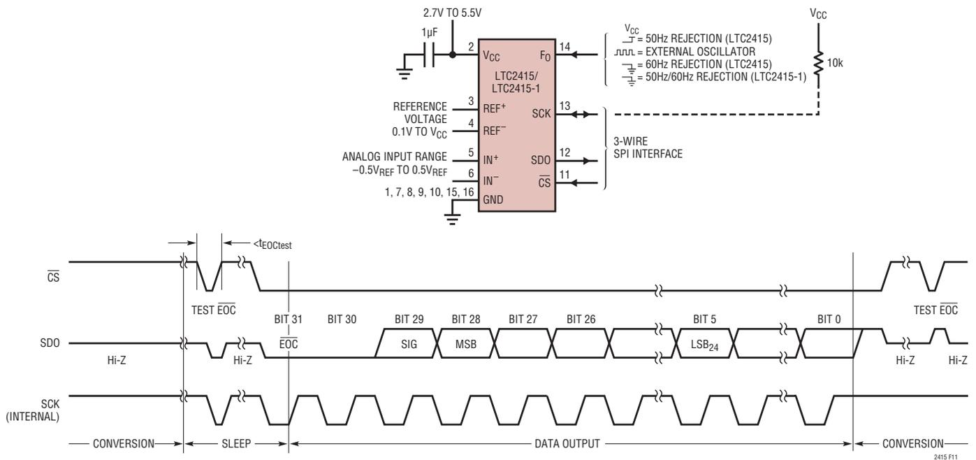
Figure 11. Internal Serial Clock, Single Cycle Operation
