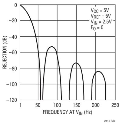
Figure 30. Rejection vs Frequency at V<sub>IN</sub>
