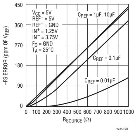
Figure 28. -FS Error vs  $R_{SOURCE}$  at REF<sup>+</sup> and REF<sup>-</sup> (Large  $C_{REF}$ )
