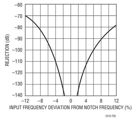
Figure 32. Rejection vs Frequency at V<sub>IN</sub>
