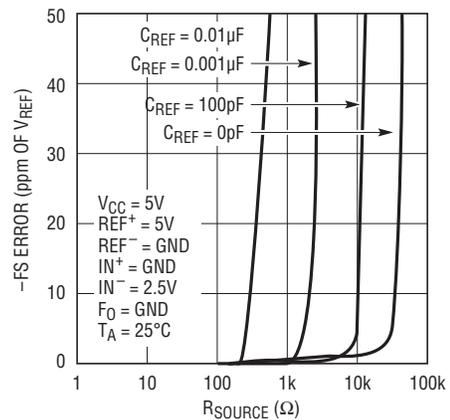
Figure 26. -FS Error vs  $R_{SOURCE}$  at REF<sup>+</sup> or REF<sup>-</sup> (Small  $C_{IN}$ )
