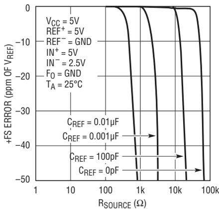
Figure 25. +FS Error vs  $R_{SOURCE}$  at REF<sup>+</sup> or REF<sup>-</sup> (Small  $C_{IN}$ )
