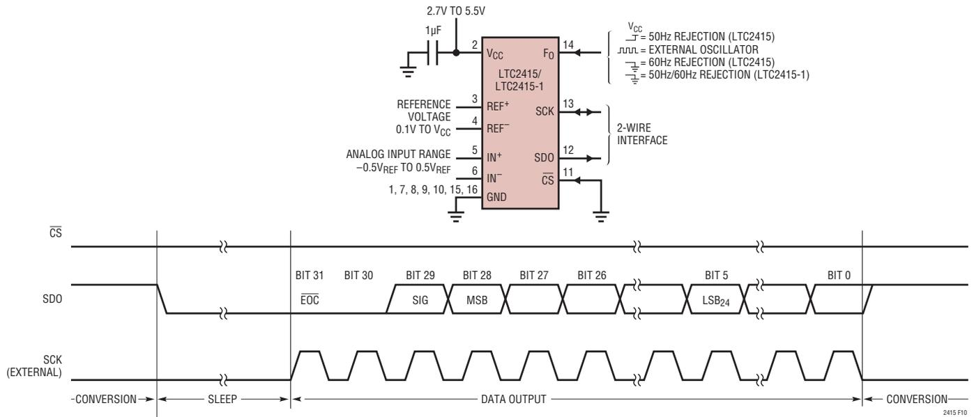
Figure 10. External Serial Clock,  $\overline{CS} = 0$  Operation (2-Wire)
