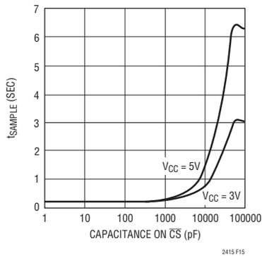
Figure 15.  $\overline{CS}$  Capacitance vs  $t_{SAMPLE}$
