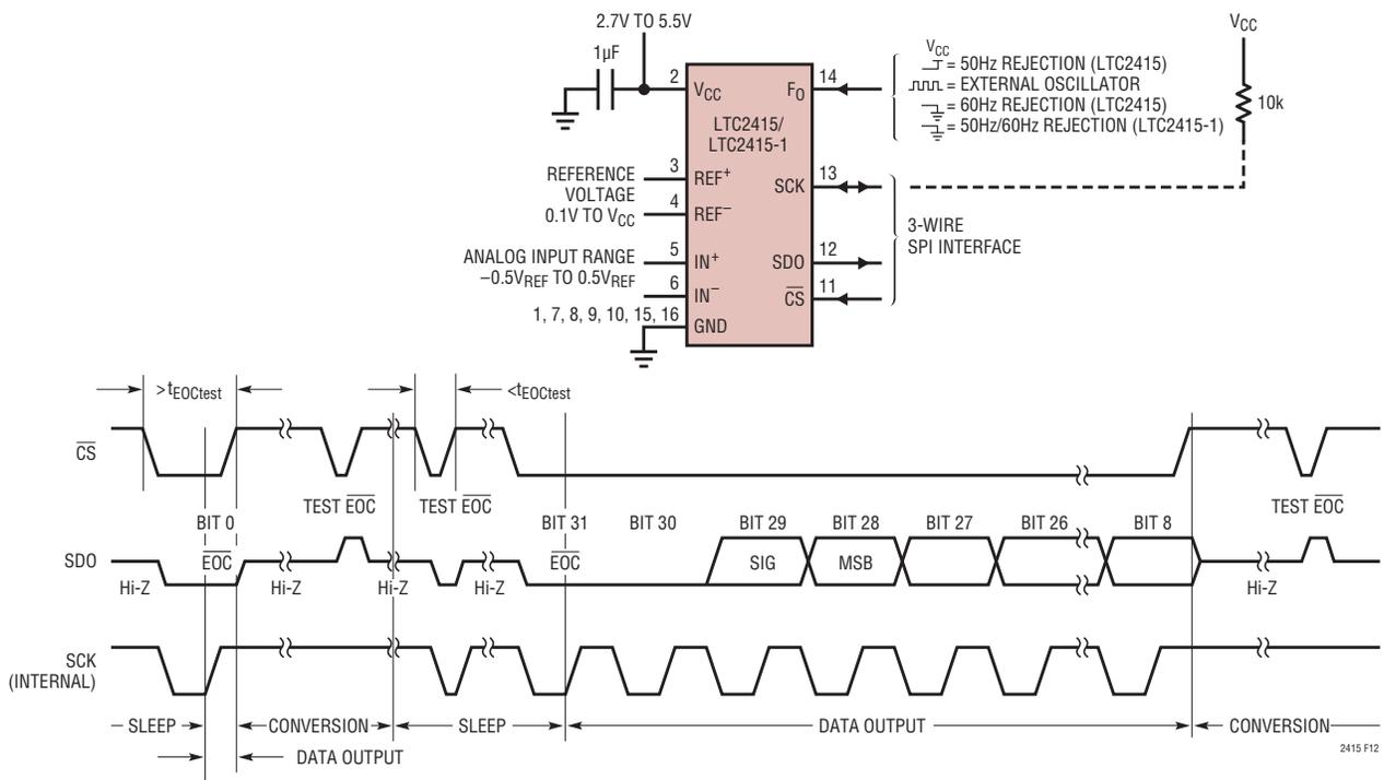
Figure 12. Internal Serial Clock, Reduced Data Output Length
