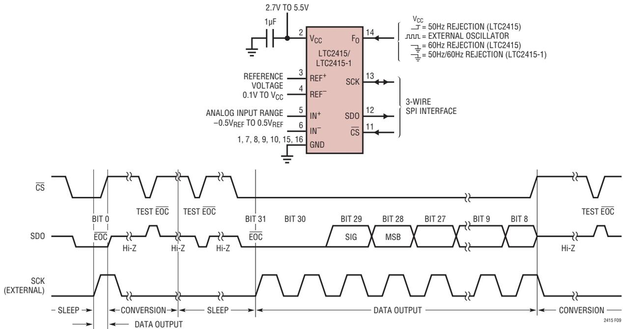
Figure 9. External Serial Clock, Reduced Data Output Length
