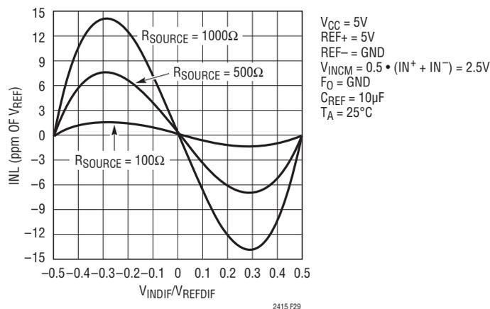
**Figure 29. INL vs Differential Input Voltage ( $V_{IN} = IN^+ - IN^-$ ) and Reference Source Resistance ( $R_{SOURCE}$  at REF<sup>+</sup> and REF<sup>-</sup> for Large C<sub>REF</sub> Values (C<sub>REF</sub> ≥ 1μF)**
