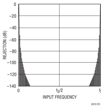
Figure 31. Rejection vs Frequency at V<sub>IN</sub>
