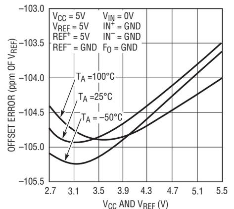
Figure 6. Offset vs  $V_{CC}$  ( $V_{REF} = V_{CC}$ )
