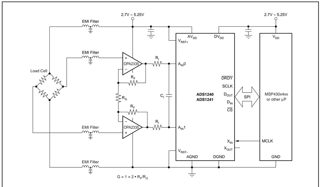
FIGURE 9. Block Diagram for a High-Precision Weigh Scale.
