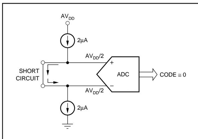
FIGURE 4. Burnout detection while sensor is short-circuited.
