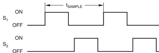
Figure 37. S<sub>1</sub> and S<sub>2</sub> Switch Timing
