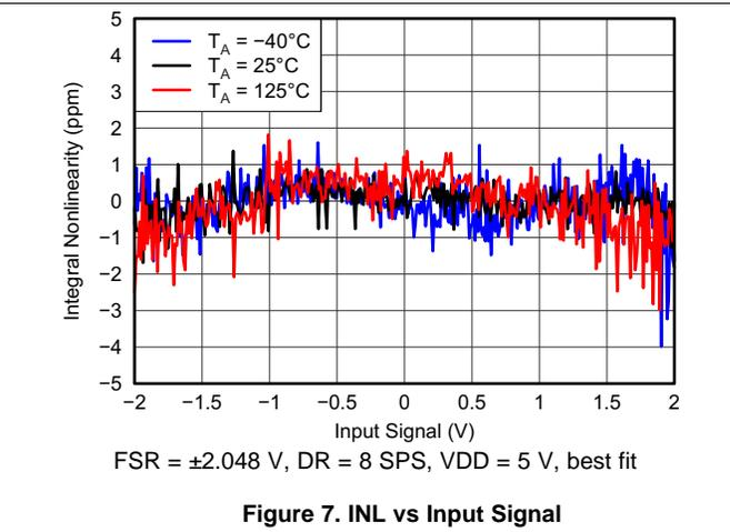
Figure 7. INL vs Input Signal
