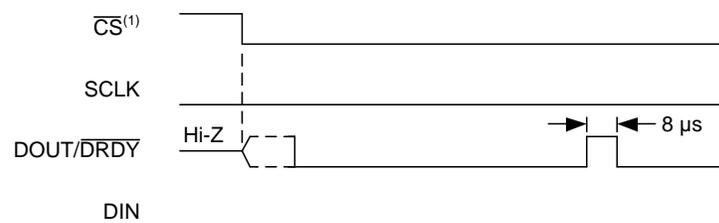
(1)  $\overline{\text{CS}}$  may be held low. If  $\overline{\text{CS}}$  is low, DOUT/ $\overline{\text{DRDY}}$  asserts low indicating new data are available.
