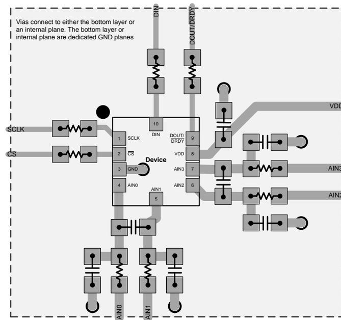
Figure 56. X2QFN Package
