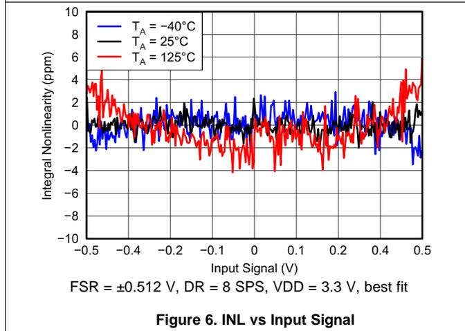
Figure 6. INL vs Input Signal
