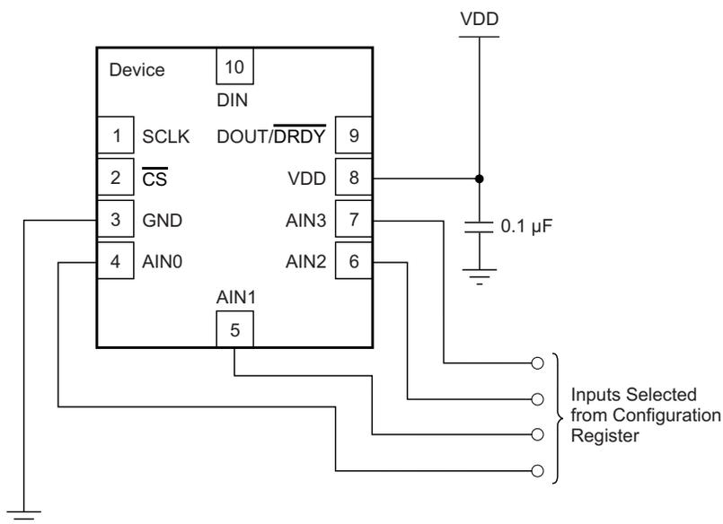
NOTE: Digital pin connections omitted for clarity.
