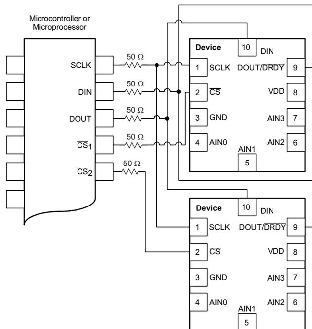
NOTE: Power and input connections omitted for clarity.
