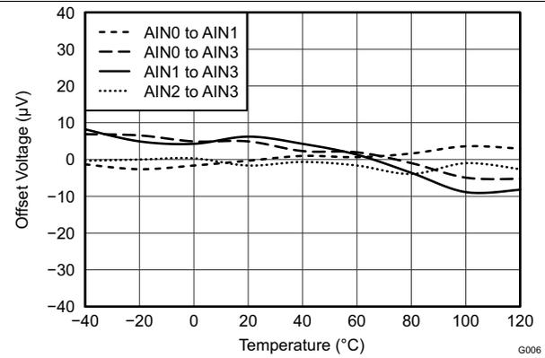
Figure 13. Differential Offset Voltage vs Temperature
