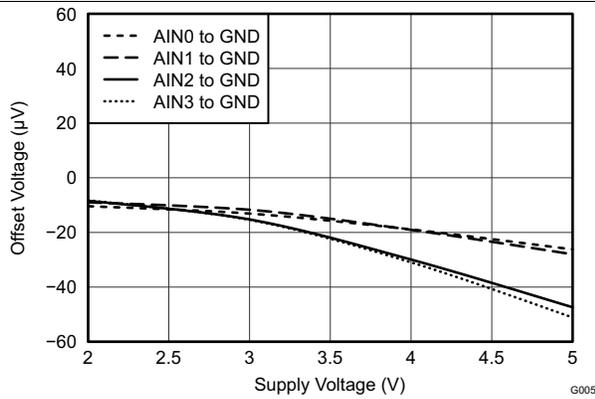
Figure 12. Single-Ended Offset Voltage vs Supply
