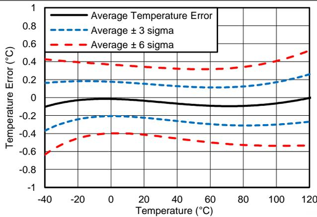
Figure 26. Temperature Sensor Error vs Temp (X2QFN)
