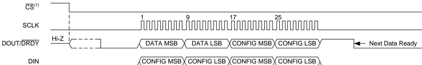
(1)  $\overline{CS}$  can be held low if the ADS1118 does not share the serial bus with another device. If  $\overline{CS}$  is low,  $\overline{DOUT/DRDY}$  asserts low indicating new data are available.
