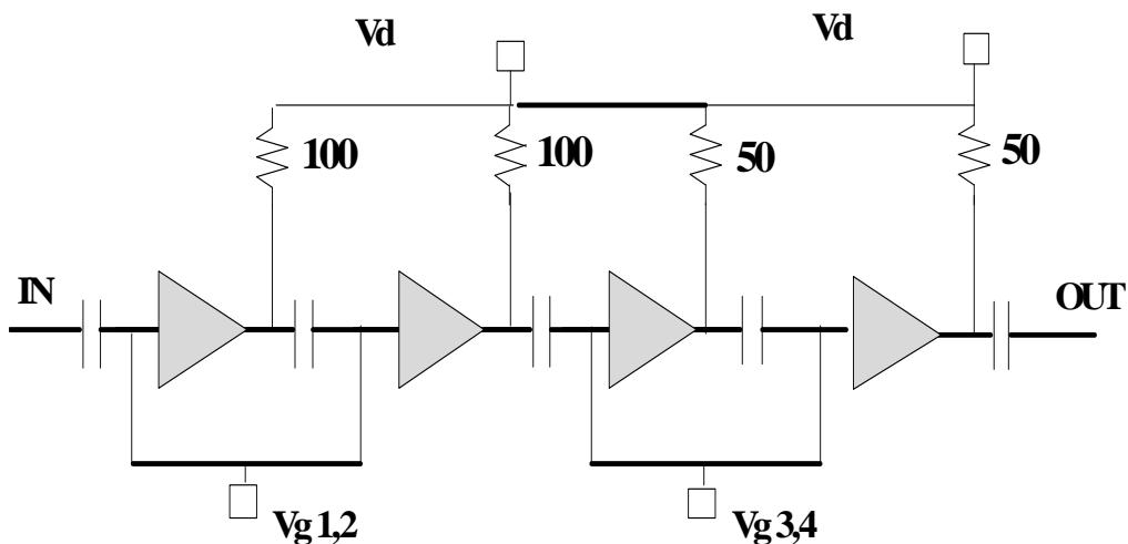
For low noise operation, a separate access to the gate voltages of the two first stages ( $V_{g1,2}$ ), and of the two last stage ( $V_{g3,4}$ ) is provided. Nominal bias is obtained for a typical current of 60 mA for the output stages and 30 mA for the two first stages (90 mA for the amplifier).
