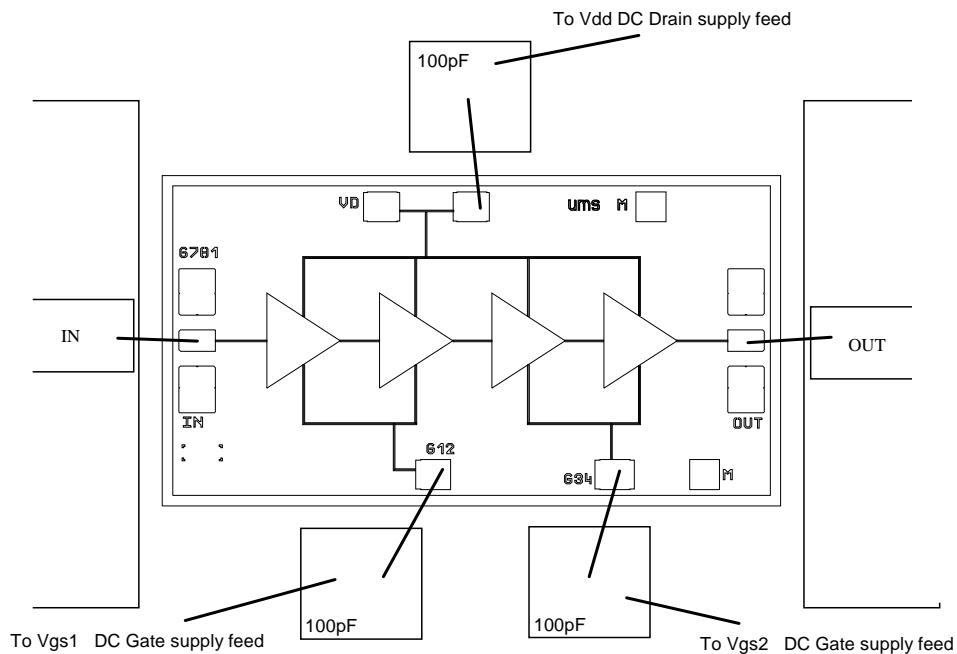
Note: Supply feed should be capacitively bypassed.
