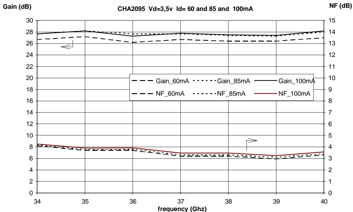
Wide band on wafer Sij parameter measurements
