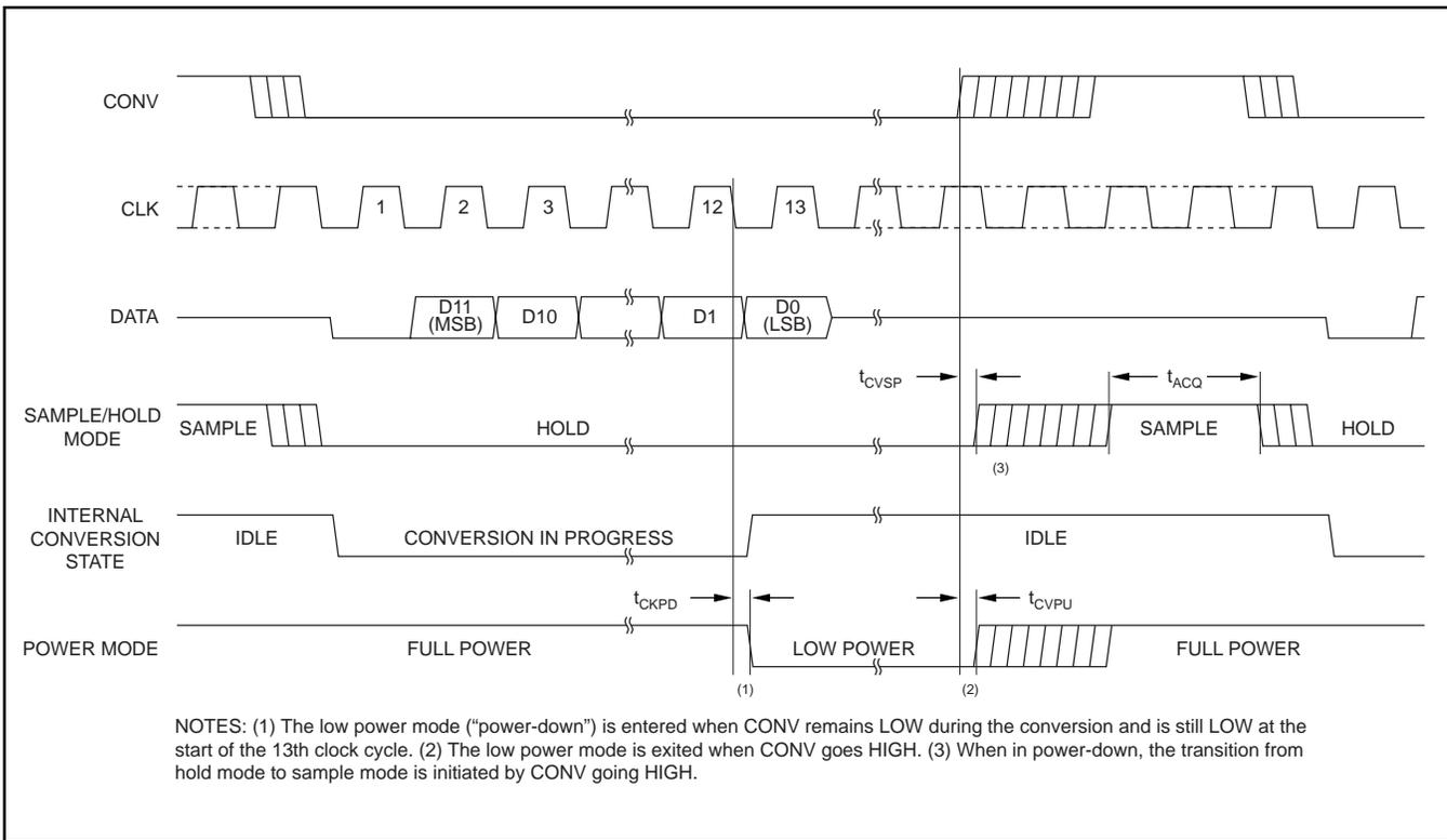
FIGURE 4. Power-down Timing.
