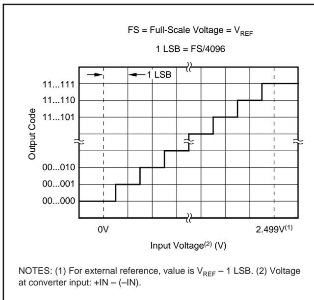
FIGURE 7. Ideal Input Voltages and Output Codes.
