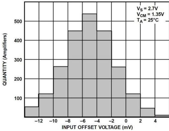
Figure 6. Input Offset Voltage Distribution Figure
