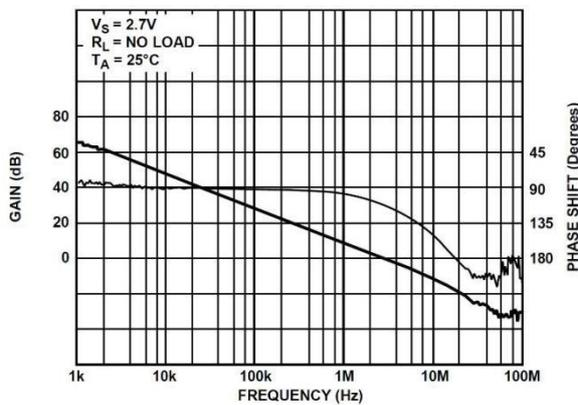
14. Open-Loop Gain and Phase Shift vs. Figure Frequency
