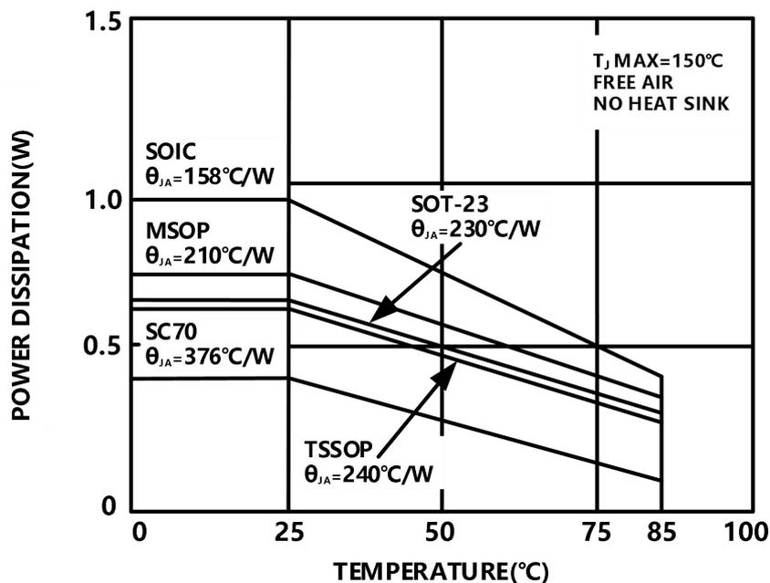
Figure 38. Maximum Power Dissipation vs. Ambient Temperature  $T_J$
