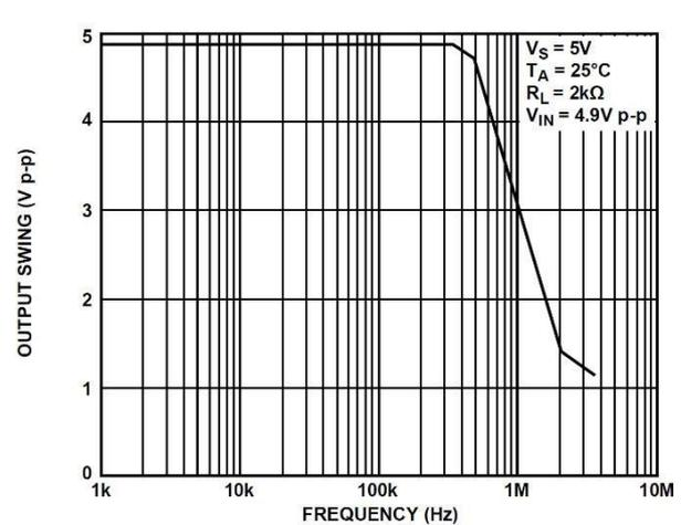
17. Closed-Loop Output Swing vs. Frequency
