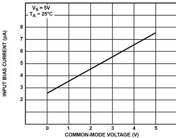
Figure 10. Input Bias Current vs. Common-Mode Voltage Figure
