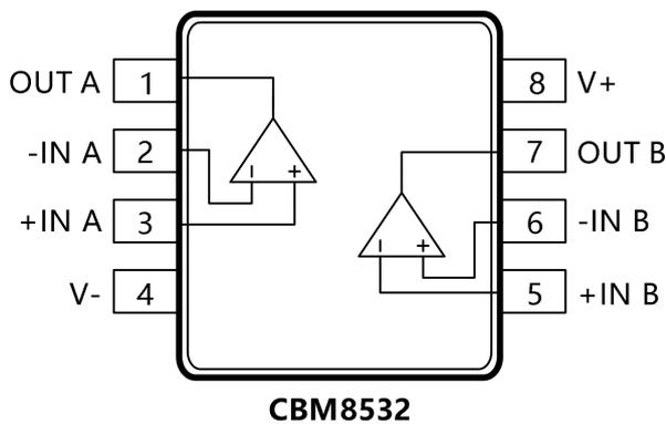
Figure 3. 8-Lead SOP, 8-Lead TSSOP-8 and
