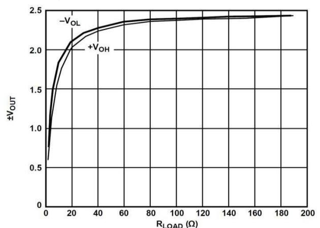
Figure 5. Output Voltage vs. Load,  $V_S = \pm 2.5V$ ,  $R_{LOAD}$  Is Connected to GND (0 V)
