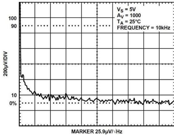
Figure 20. Voltage Noise Density vs. Figure Frequency (10 kHz)
