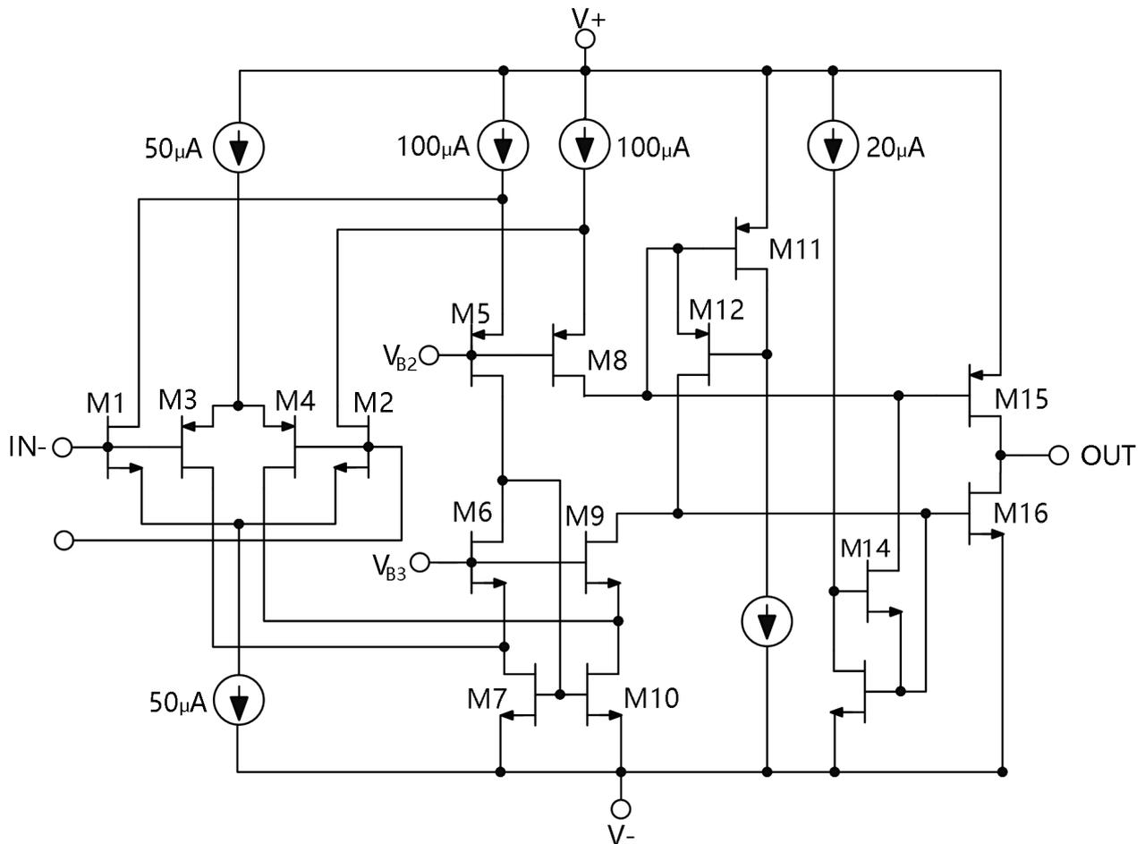
Figure 36. Simplified Equivalent Circuit
