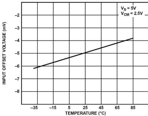
Figure 8. Input Offset Voltage vs. Temperature Figure
