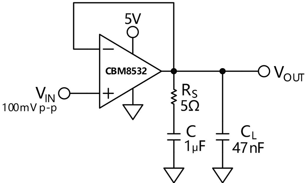
Figure 40. Snubber Network Compensates for Capacitive Loads
