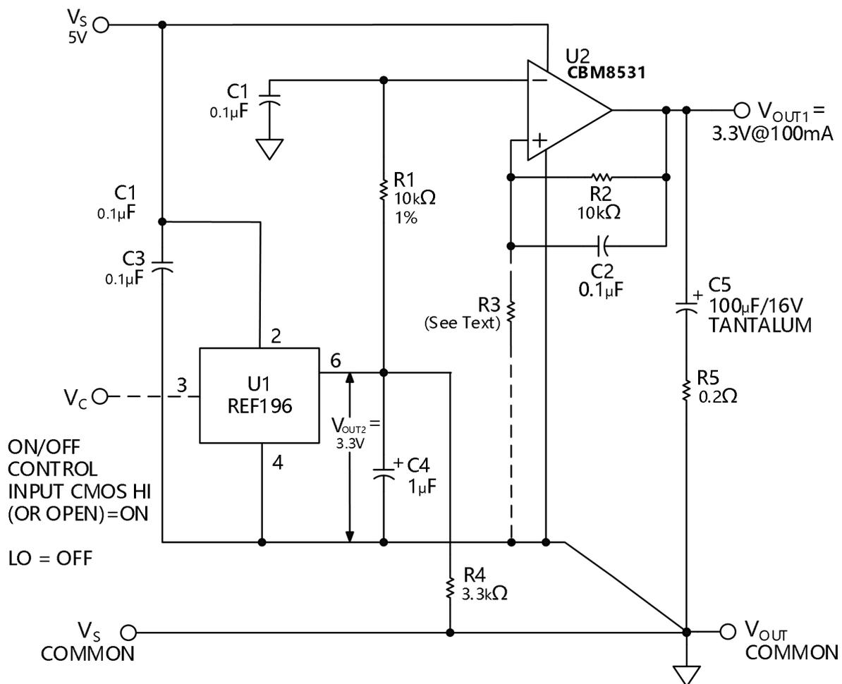
Figure 42. High Output Current Reference/Regulator
