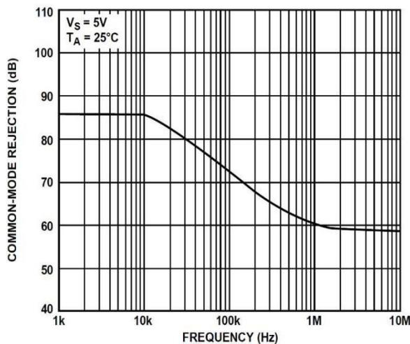
Figure 22. Common-Mode Rejection vs. Frequency Figure
