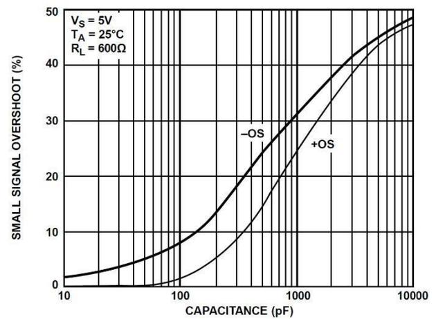
27. Small Signal Overshoot vs. Load Capacitance
