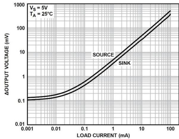
13. Output Voltage to Supply Rail vs. Load Current
