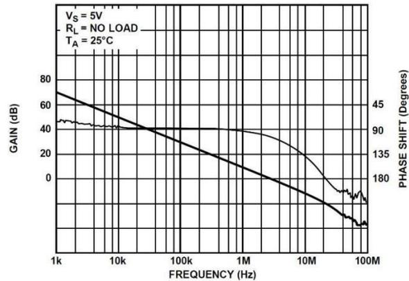
15. Open-Loop Gain and Phase Shift vs. Figure Frequency
