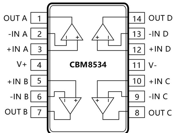
Figure 4. 14-Lead SOP and
