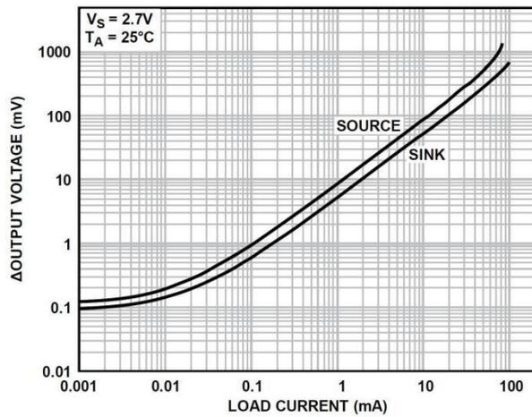
Figure 12. Output Voltage to Supply Rail vs. Load Current Figure
