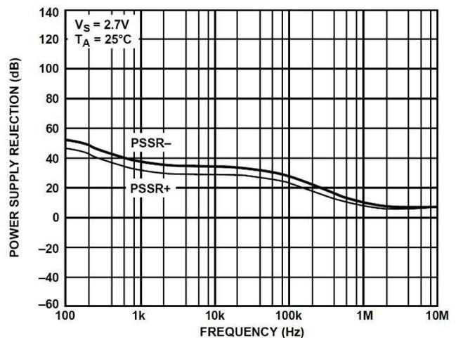
23. Power Supply Rejection vs. Frequency
