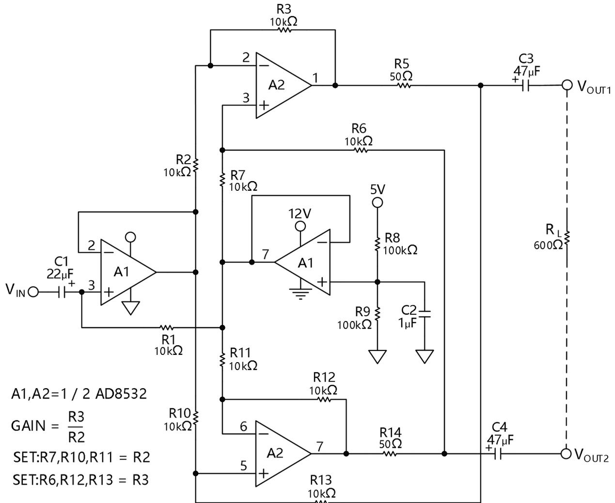
Figure 43. Single-Supply, Balanced Line Driver for Multimedia and Automotive Applications
