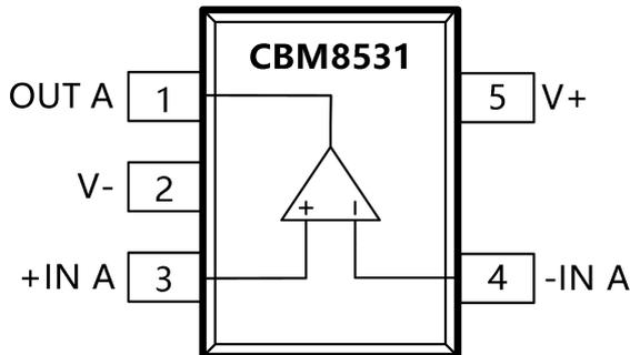
Figure 1. 5-Lead SC70 and 5-Lead SOT-23
