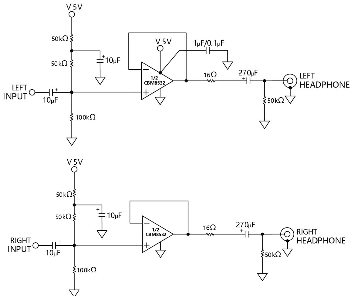
Figure 44. Single-Supply, Stereo Headphone Driver
