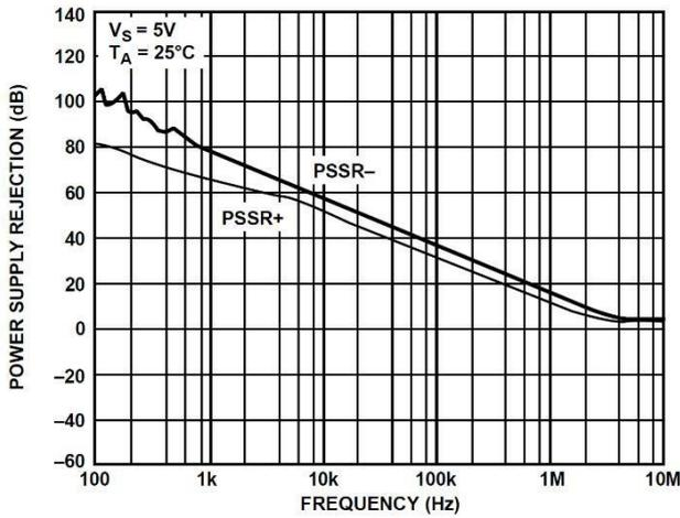
Figure 24. Power Supply Rejection vs. Frequency Figure
