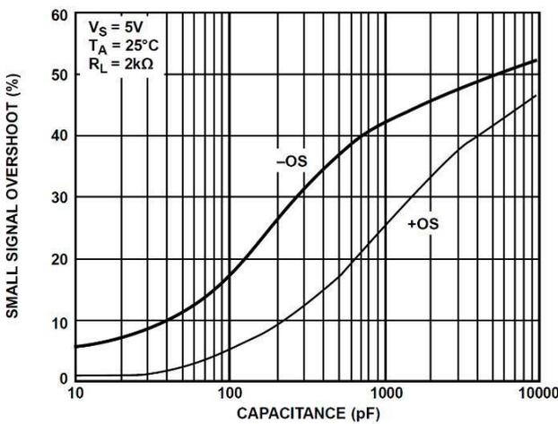
Figure 26. Small Signal Overshoot vs. Load Capacitance Figure
