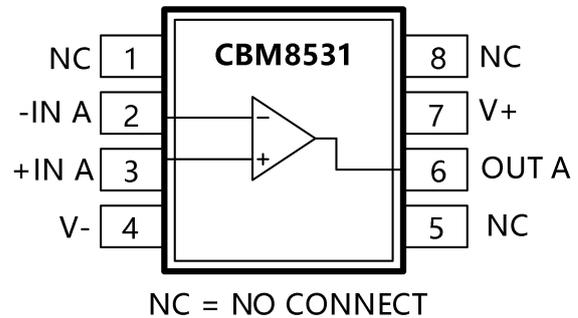
Figure 2. 8-Lead SOP (R Suffix)
