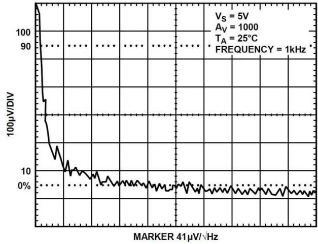
19. Voltage Noise Density vs. Frequency (1kHz)
