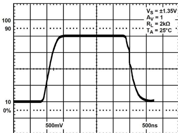
Figure 34. Large Signal Transient Response Figure
