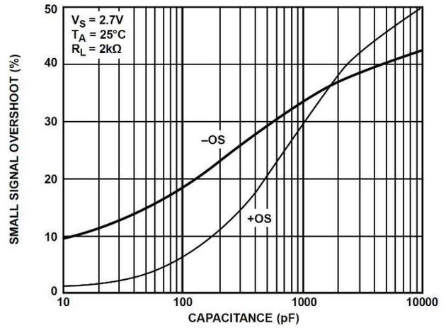
25. Small Signal Overshoot vs. Load Capacitance
