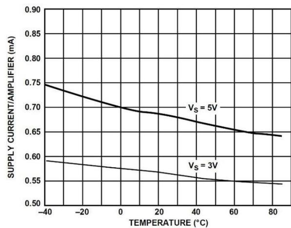
29. Supply Current per Amplifier vs. Figure Temperature
