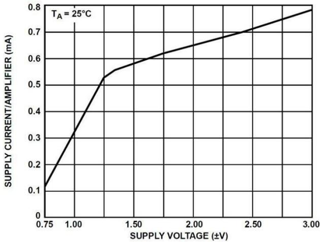
Figure 30. Supply Current per Amplifier vs. Supply Voltage Figure
