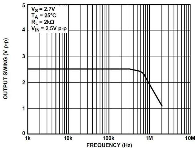
Figure 16. Closed-Loop Output Swing vs. Frequency Figure
