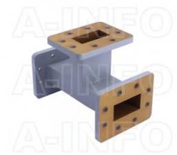
159WET WR159 Waveguide E-Plane Tee 4.9-7.05GHz with Three Rectangular Waveguide Interfaces
